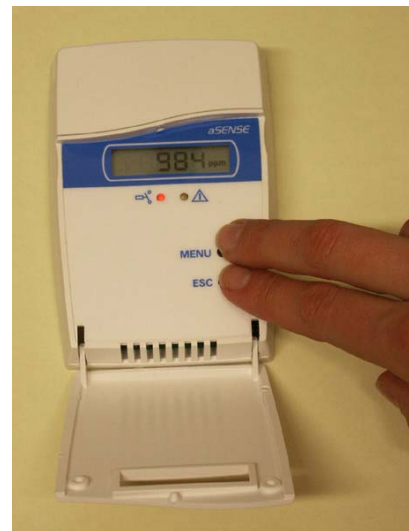
The ENTER command is done by pushing buttons MENU and ESC at the same time for about 14 seconds
